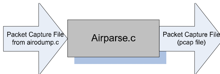
Figure 8 – Airparse.c Input/Output Sequence
